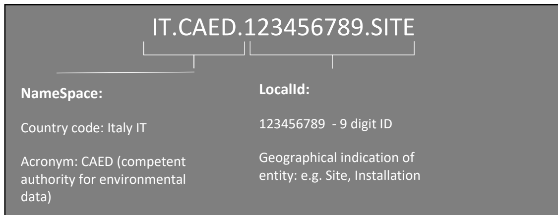
Figure 4 - An example inspireId broken into its components.
